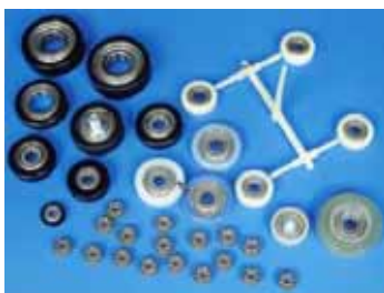
Injection molding (bearing, etc.)
